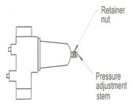
In some cases the internal components of the pressure regulator may need to be cleaned, to perform this procedure please refer to the manufactures recommended maintenance instructions or contact a licensed plumber. If you chose to perform maintenance on the pressure regulator such as cleaning of the internal seats and screens be sure to shut the water off before the regulator before you proceed.
